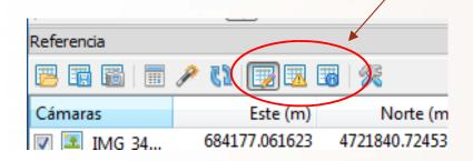
39. Projections. One of the columns in the Reference Pane (marker zone) is Projections. Projections are the number of measured photos in a GCP. The higher the number of projections the greater reliability of that GCP.
