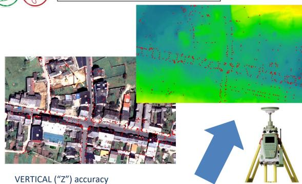
X,Y,Z data measured with TOTAL STATION, GPS
